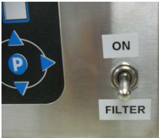
Right Controller showing On/Off toggle switch. In the up (on) position the controller is turned on. In the down (off) position the controller is turned off and the filtration circuit is activated.
