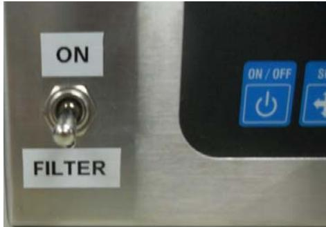
Left Controller showing On/Off toggle switch. In the up (on) position the controller is turned on. In the down (off) position the controller is turned off and the filtration circuit is activated.
