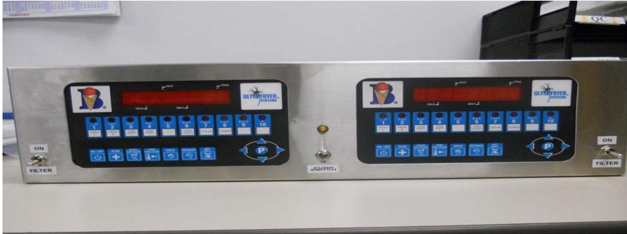
**PURPOSE:** Position #4 (USTAT) provides power to the primary control box containing the U-23 controllers. This position is the standard position to operate the fryer.
